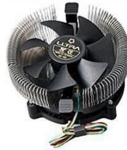
(CPU fan with heat sink)
